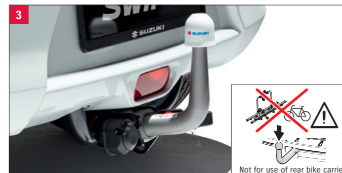
3 | Tow Bar 2 WVTA Detachable, for trailers only. The max vertical load : 60kg The max towing capacity : 1,000kg Part No. 72901-53R02-000 F G H I J K
